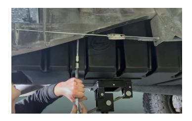
Install the S&B support bar in front of the S&B Tank. The hooks should be over the inside lip of the frame rail. Then by pressing up on the tank and pushing on the bar, slide the bar under the S&B Tank until it is in the groove on the S&B Tank.
