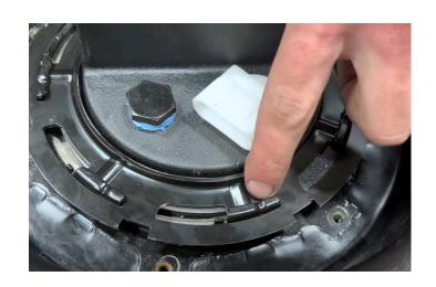
Transfer the feed and return line from the OEM tank to the S&B Tank
