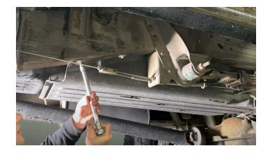
With fuel line disconnect tools, disconnect the fuel feed and return lines above the fuel cooler.
