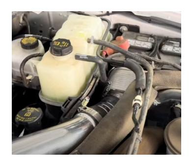
Install the Christmas tree clip into the bracket and reconnect the sensor.
