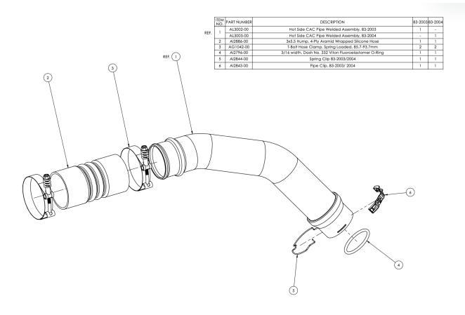
Start by loosening the hose clamp on the intercooler side.
