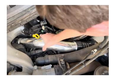
Using an 11mm, remove the nuts on the springs in order to make them easier to install.
