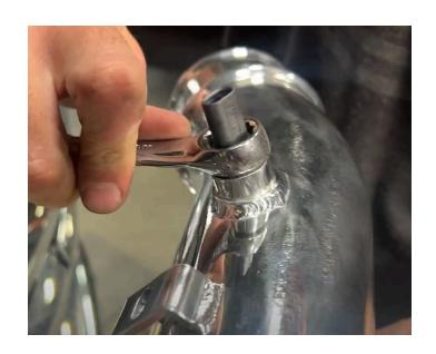
Slightly slide the S&B intercooler onto the collar at the turbo.
