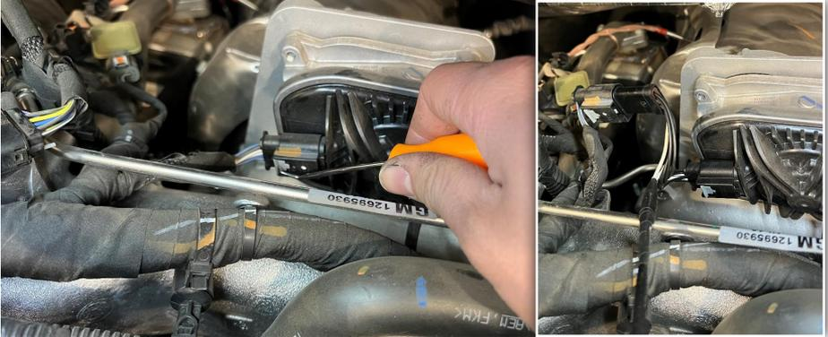
**STEP 6** - Clean the fuse box lid that's right in front of the coolant reservoir. Connect the EZ harness to the EZ module and secure the module to the fuse box using the supplied Velcro strips.
