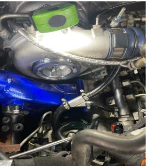
We run the fuel in from the quick disconnect (12-16 MY) or fuel pipe with hose clamp (2011 MY), to the WYE fitting, which connects to the Drivers fuel rail return nipple and then runs either to the  $\frac{1}{2}$ " feed fitting on the pump (for lift pump applications), or to the filter head connection on the passenger side if retaining the factory filter head.
