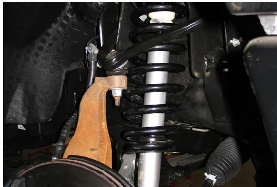
29. Attach the lower strut mount to the lower control arm, torque the lower strut nut and bolt to 351 ft lbs.
