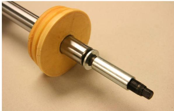
24. With the OEM spring still compressed, slide the new Belltech strut into the OEM spring and install Belltech bump stop on the strut rod.
