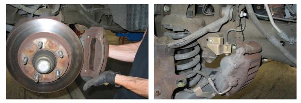
10. Remove the hub and rotor assembly from the spindle by removing the grease cap, cotter pin, spindle nut, and washer from the spindle pin. Carefully slide the rotor assembly off the spindle pin, do not let the outer bearing fall out of the hub.
