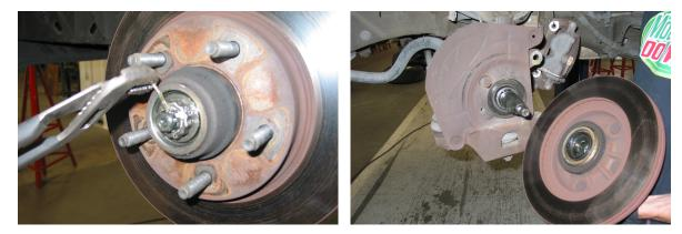
11. Remove the three 8mm bolts from the dust shield. Detach the shield and gasket from the face of the spindle.
