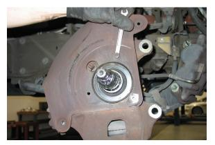
12. Remove the 8mm bolt from the wheel sensor at the steering spindle. Detach the clip holding the sensor line to the upper control arm. Place the sensor away from the work space.
