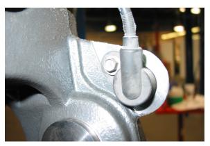
23. Place the gasket and dust shield onto the face of the spindle. Secure the dust shield with the original bolts; torque to 9 ft lbs.
