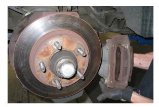
28. Rotate the steering spindle in both directions to check if the brake line and sensor cable have proper clearance. If needed, adjust as necessary.
