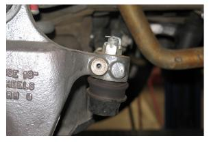
22. Attach the wheel speed sensor to the spindle with the original bolt. Ensure the sensor is free from dirt or grease before installation.
