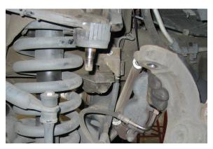
16. Remove the 24mm lower control arm ball joint nut. Use a puller tool to detach the ball joint from the spindle. Alternatively, you can leave the nut on the ball joint and strike the spindle with a hammer to dislodge the ball joint. Do not hit the boot.
