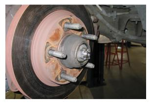
27. Use the original bolts to attach the brake caliper assembly onto the spindle. Torque the two bolts to 150 ft lbs.
