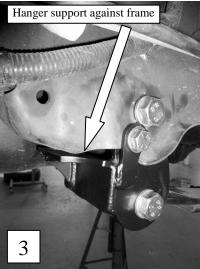
2c) Clamp the hanger into place or have an assistant hold the bracket in place during drilling to ensure the hole location does not move. Drill a ½" hole centered in the hole of the locating tab. (**Photo 2**) Drill all the way through both sides of the original bracket.
