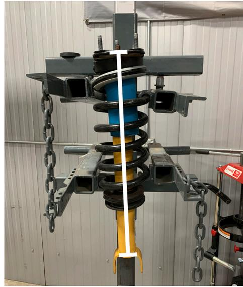
19. Compress the spring until tension is relieved from the strut.
