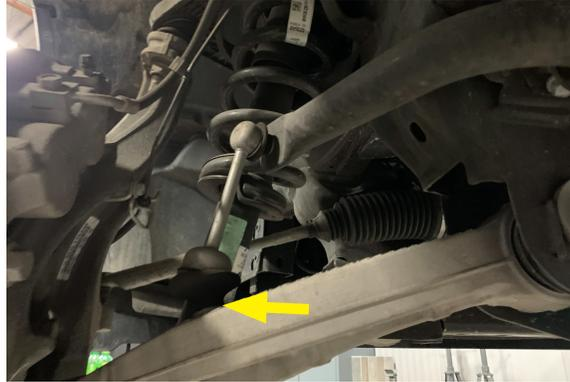
10. Remove the tie rod nut from the spindle. Strike the side of the mount with a dead blow hammer or use a puller to dislodge the tie rod end.
