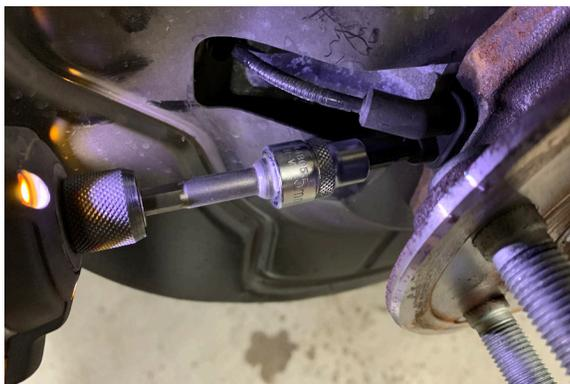
39. Attach the outer tie rods into the spindle. Torque to 41 ft lbs. + 180° turn.
