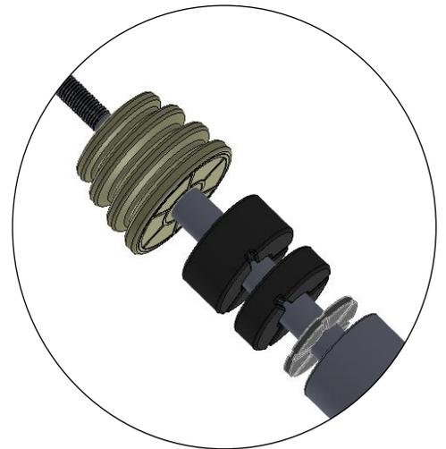
25. With the OEM spring still compressed, slide the new Belltech strut into the OEM spring and install Belltech bump stop on the strut rod.
