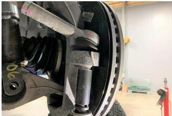
11. Remove all mounting points for the brake line and ABS sensor wire from the upper control arm and spindle.
