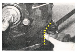
21. Mount the hub and rotor assembly onto the new spindle by reversing the procedure of removal in Step 10. Add grease to the new spindle pin. Torque the spindle nut to 25 ft lbs. and rotate the hub to ensure the bearings are seated. Back the spindle nut off and tighten by hand so that there little drag.
