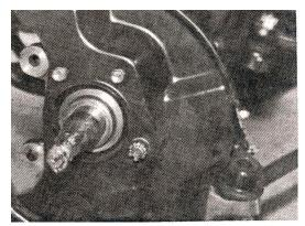
11. Remove the cotter pin from the 19mm nut on the tie rod end. Loosen the nut, but don't remove it completely. Use a tie rod puller or use a hammer to strike the side of the steering arm until the tie rod end is dislodged; swing the rod out of the way.
