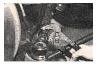
24. Mount your wheel and tire combination onto your truck. Place the original steering stop on the new spindle. Turn the wheel by hand to make sure there are no clearance problems. Turn the wheel completely right to left and set the steering stop to ensure the wheel and tire do not contact any components. Depending on your wheel choice, some slight grinding of the lower control arm may be necessary.
