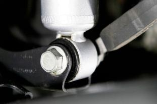
15. Install the rear Belltech shocks with the original upper bolts, torque to 37 ft lbs. Attach the lower shock eyelets to the axle using the original nut and bolt. Torque to 65 ft lbs.
