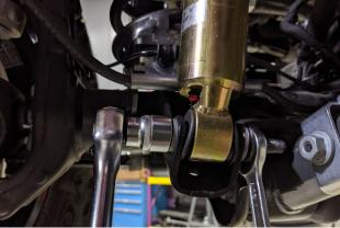
16. Install the rear Belltech shocks attaching the shock eyelets to the upper mount and axle using the original nuts and bolts. Torque to 80 ft lbs.
