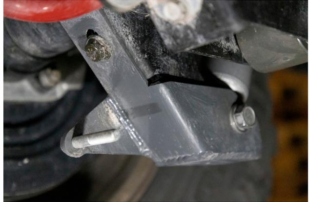
23. Adjust end link lengths as necessary to hold the sway bar arms as parallel to the ground as possible; then tighten the jam nuts.
