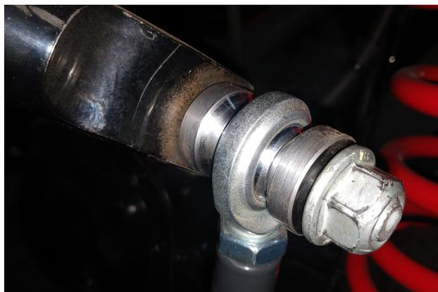
15. Assemble the front passenger side quick release clevis pin with a spring washer as shown.
