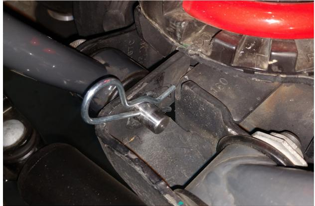
17. Slide the driver side end link onto the pin on the axle, and secure with cotter pin.
