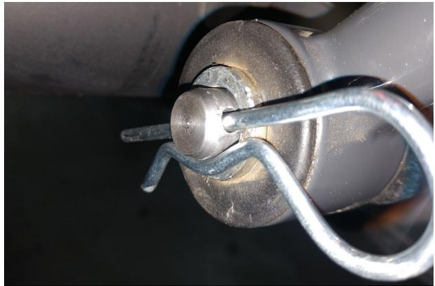
18. Adjust end links to the desired length. Tighten jam nut while keeping the Heim joint centered.
