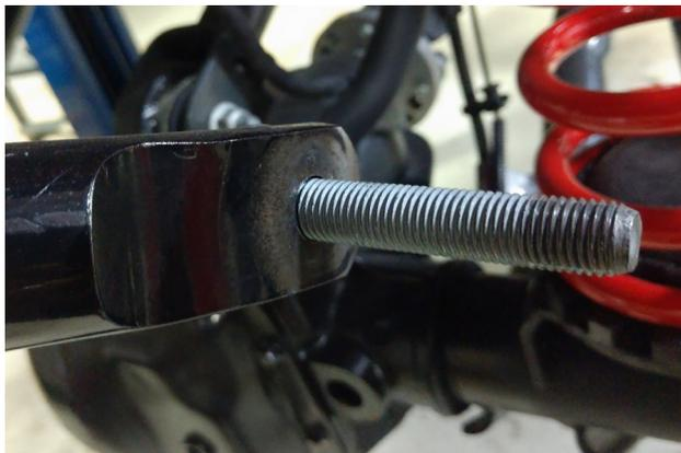
14. Install the new front end links with a cone spacer on each side of the upper Heim. Use the original lower nut on the drivers side. On the passenger side, use the supplied nylon lock nut. Torque the upper nut to 69 ft lbs. Leave the jam nut on the end link loose at this time.
