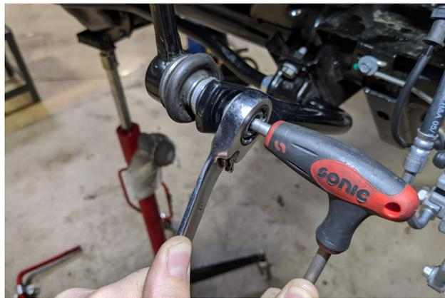
21. To install the end link disconnect holder brackets, remove the lower shock bolt, and swing the shock out of the way. Attach the bracket to the lower shock mount; place the M12 x 1.75-25mm bolt through the existing hole in the lower shock mount and fasten the bolt with the M12 flag nut from inside the lower shock mount. Leave the bracket loose until the shock hardware is tightened.
