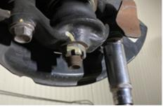
12. Remove the bolt and nut securing the lower shock eyelet to the lower control arm.
