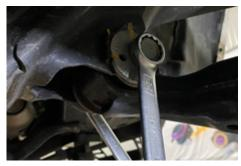
15. With the lower control arm swung out of the way, the strut should be held only by the three nuts on the top mount. While holding the strut up to avoid dropping it, loosen and remove the top three nuts using a 14mm wrench.
