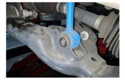
13. Using an oil-based paint pen, mark the alignment of the camber and caster adjustment bolts securing the lower control arm to the frame. When reinstalling the control arms later, this will help keep the alignment close to proper settings.
