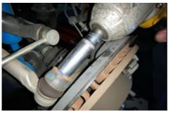
11. Using a 19mm socket, remove the two bolts securing the lower ball joint to the spindle. Be careful to stabilize the spindle as it may now move freely.
