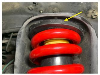
29. Torque the supplied nylock nut onto the strut. Reference the OE strut markings and ensure the top mount is oriented in the same fashion it was before disassembly.
