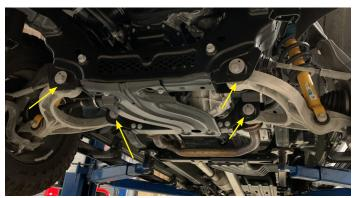
10. Use an 18mm socket to remove the sway bar end links.
