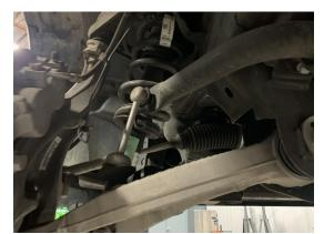
11. Remove the bottom OE strut fork bolt using both a 21mm and a 24mm wrench.
