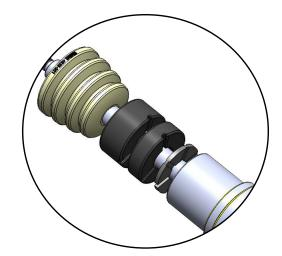
23. Confirm the vent disk is located on the strut, under the dust boot. If for any reason your vent disk is not present, please call our technical support staff before proceeding, as driving on the strut without it could cause the shock to fail.
