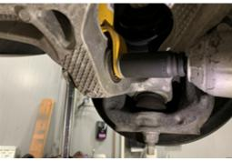
12. Swing the control arm down and away from the strut.
