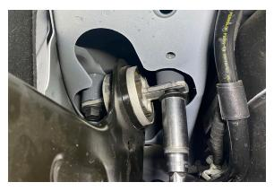
35. Attach the original lower coil spring pad to the Belltech rear lift spacer. Align the locator pin on the original spring pad with the hole in the lift spacer.
