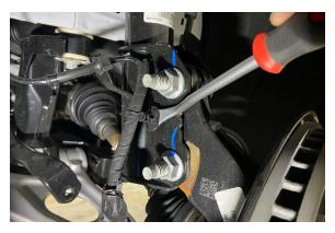
13. Remove the 8mm brake line mount bolt to detach the line from the strut.
