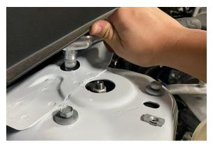
17. The lower back side of the struts will need to be trimmed to create clearance for the axle under full droop. Mark the area as shown in the image; trim it using an angle grinder. Ensure not to grind too much to prevent compromising the structure of the damper. Upon installation, turn the knuckle both ways under full extension to determine if more trimming is needed.
