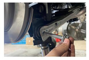
31. Break loose the upper control arm and front lower bolts but do not remove them. This allows the trailing arm, hub, and brake assemblies to droop further.
