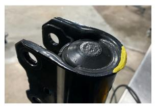
18. After the strut is trimmed, it should look similar to the image below. The trimmed surface must be coated and protected to prevent corrosion with a weather resistant spray paint.
