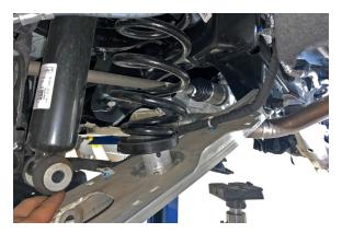
33. With the suspension loosened, it is easier to work on the front trailing arm mounts. Ensure the trailing arm is supported and will not swing or fall causing injury or damage. Remove the 15mm bolts and lower the trailing arm.
