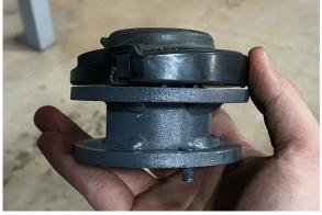
36. Install the rear Belltech lift spacer and original spring pad assembly on the lower control arm with the locator pin on the spacer in the control arm hole. Place the coil spring in the original positions marked on the upper and lower spring pads.
