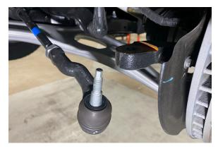
11. Remove the upper and lower 18mm end link nuts. Use a T40 Torx socket to hold the stud if needed. Detach the end link assembly from the vehicle.
