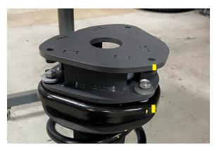
20. Place the strut and spacer assembly in the strut tower and fasten the top of the strut to the vehicle using the supplied M8 x 1.25 - 20mm bolts. Torque to 26 ft lbs.
