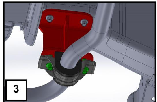
4. Do **NOT** torque down the sway bar bracket to the BELLTECH swaybar drop down bracket as it will be easier to install the rest of the components in the lift kit.
