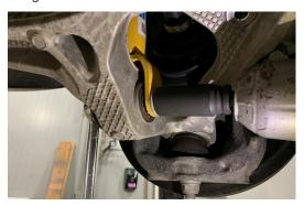
12. Swing the lower control arm down and away from the strut to separate the OEM strut from the lower control arm.
