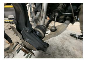
11. Remove the bottom OE strut fork bolt using both a 21mm and a 24mm wrench.
