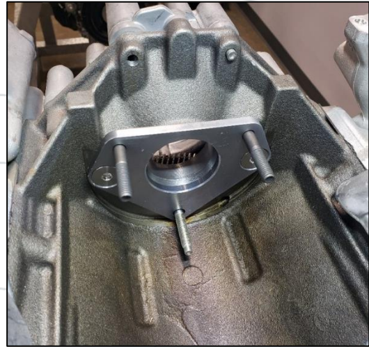
Figure 24: Engine Adapter Plate Installation on Engine Block
