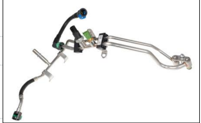
Figure 14: Low Pressure Fuel Line Assembly
